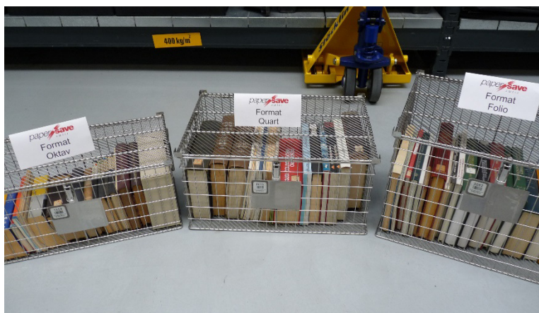
Figure 4. Selection of books and their placement in cages for PaperSave Swiss deacidification technology.
