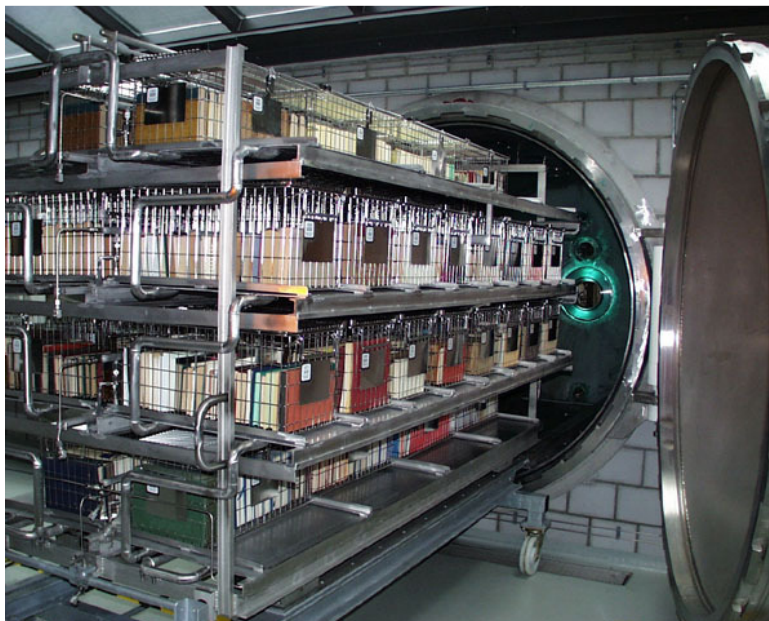
Figure 5. PaperSave Swiss ® mass deacidification technology. Source Nitrochemie.
