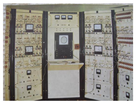
Figure 2. Repetitive Differential Analyzer
